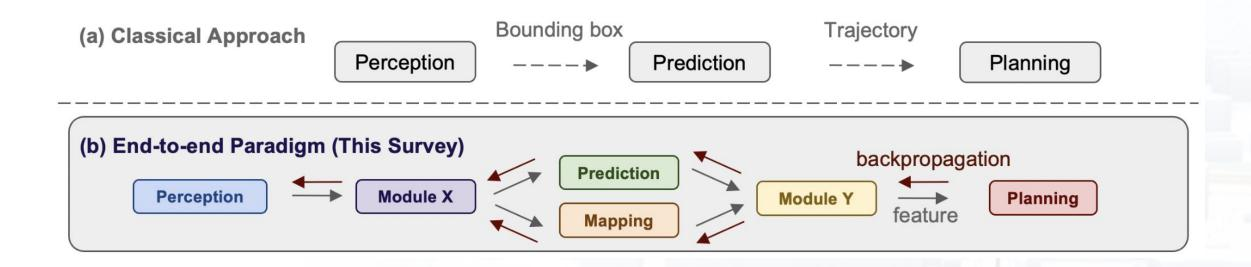
End-to-end autonomous driving system - A suite of fully differentiable programs that:
